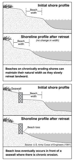
impoundment mauka (landward) of a seawall is a contributing factor to chronic  $erosion^{14}$ . Fletcher et al., found that on Oahu, 17.3 ±1.5 km (10.7 miles) of beach has been narrowed
